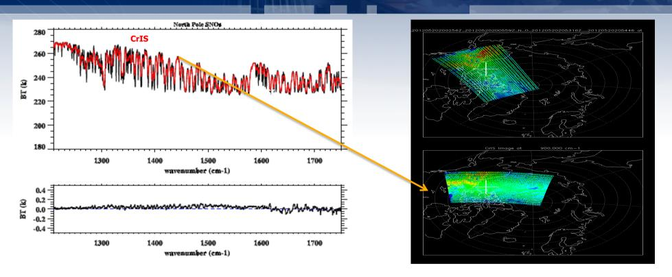
For band 2 at water vapor absorption region, CrIS and IASI are consistent to each other and the difference is close to a zero line. CrIS and IASI are nearly benchmark quality measurements and are critical for vicarious calibration of other infrared sounder and imager measurements.
